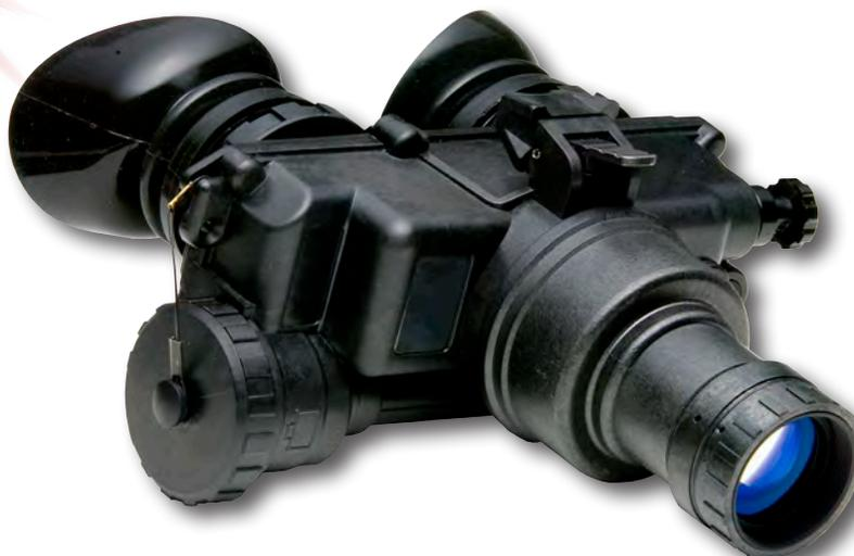
The NL963B™ night vision goggles are based on the US military model AN/PVS-7. The NL963B™ is intended for land use including vehicle driving, and is typically worn on a head mount or helmet mount. When using the helmet mount, the goggle will automatically shut off in the up position. The goggle and its adaptor are independently removable from the helmet strap. An ON-OFF knob controls all of the features of the goggle. These controls can easily be operated using gloves.
